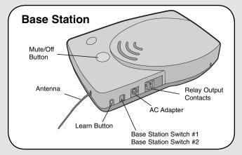
**On/Off:** To turn Base Station off hold down the Mute Button until it powers down. The Base Station can be turned on by pressing the Mute Button.
